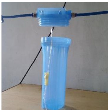
Fig.2.a: Photographic view of External MQL Set- up
