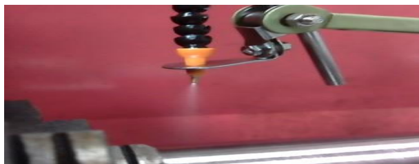
Fig.2.c: MQL Nozzle supplying mist
