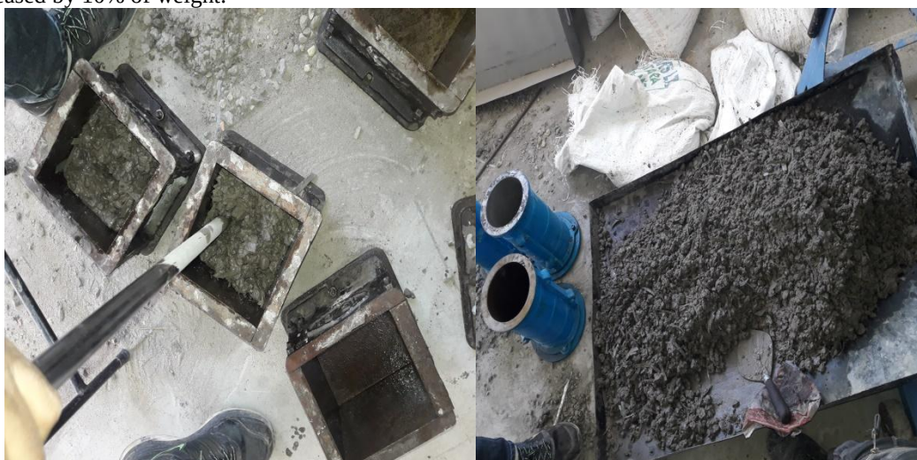
Figure.4. Casting of Specimens
