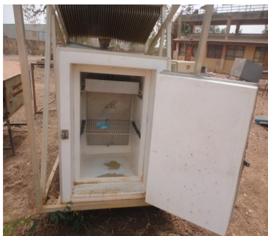
Figure 1 : Photo of the evaporator and the chest
