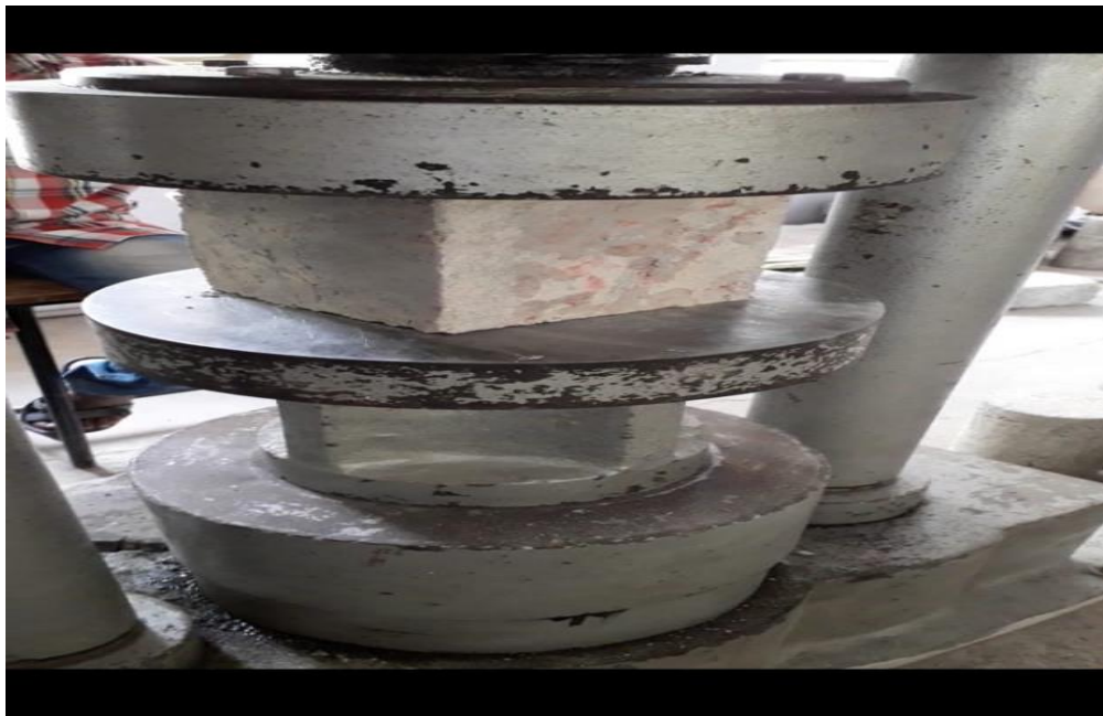
Fig. 2: Compressive strength testing set up
