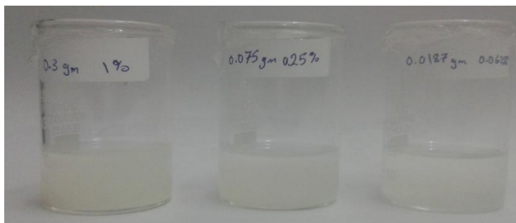
Fig. 5. Stability assessment of WO 3 /SDS nanofluids
