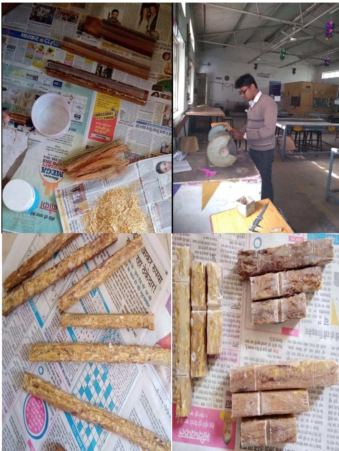
Figure 2.3 Open mould system used for making composites & Sample Preparation
