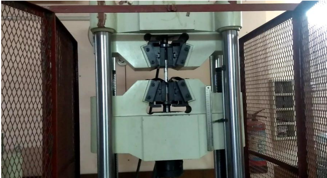
Fig.6. Setup of tensile testing
