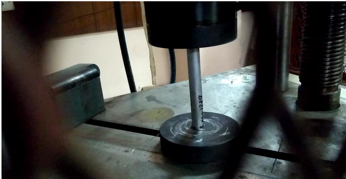
Fig.2. Setup of compressive testing
