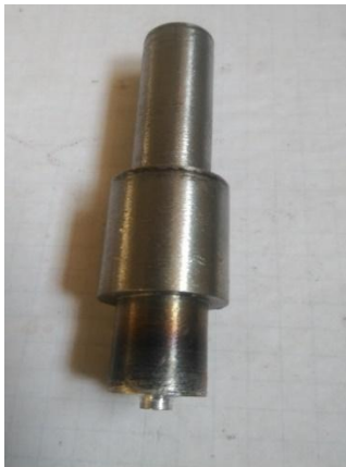
Figure: 3.2.1 FSW circular pin profile
