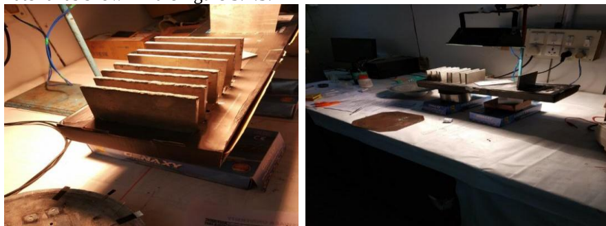
Figure: 3.1.3 drying of the magnesium coating under the solar lamp
