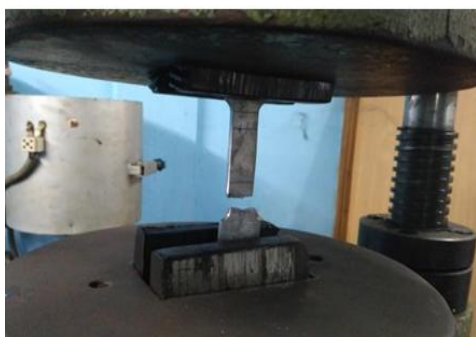
Figure: 3.3.2.4: Testing of Specimen in UTM
