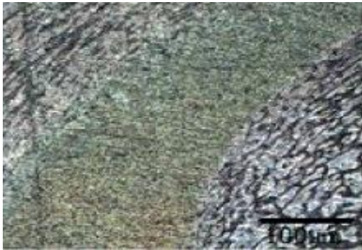
(a) Micro structure (0.25gm of mg, 40 mm/min Feed, 1000 RPM)
