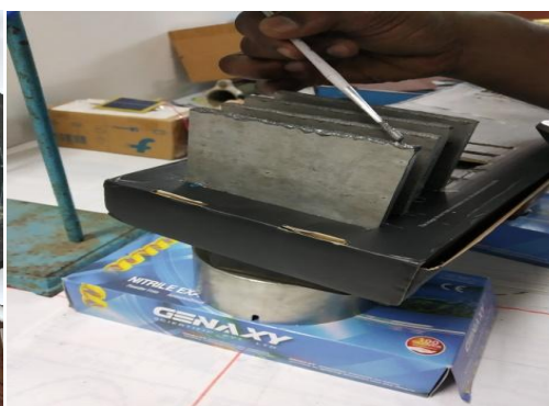
Figure: 3.1.2 Coating of the magnesium slurry on the base metal
