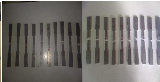
Figure: 3.3.2.5 (a & b): specimen before & after testing
