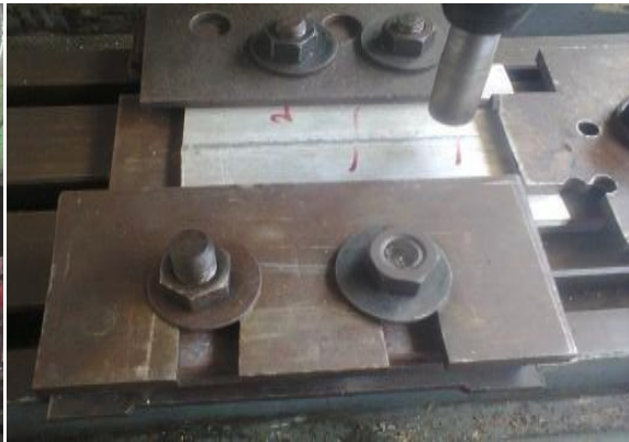
Fig. 3.1.5: Fixture setup on milling machine
