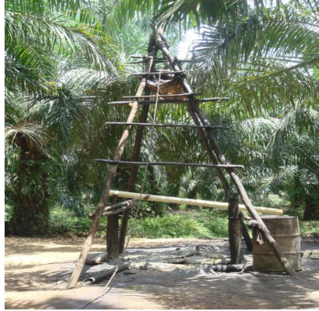
Well Service Hoist
